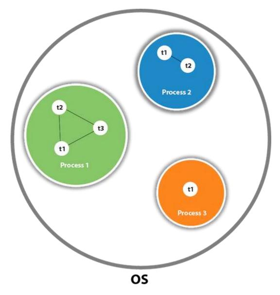
As shown in the above figure, a thread is executed inside the process. There is context-switching between the threads. There can be multiple processes inside the <u>OS</u>, and one process can have multiple threads.
